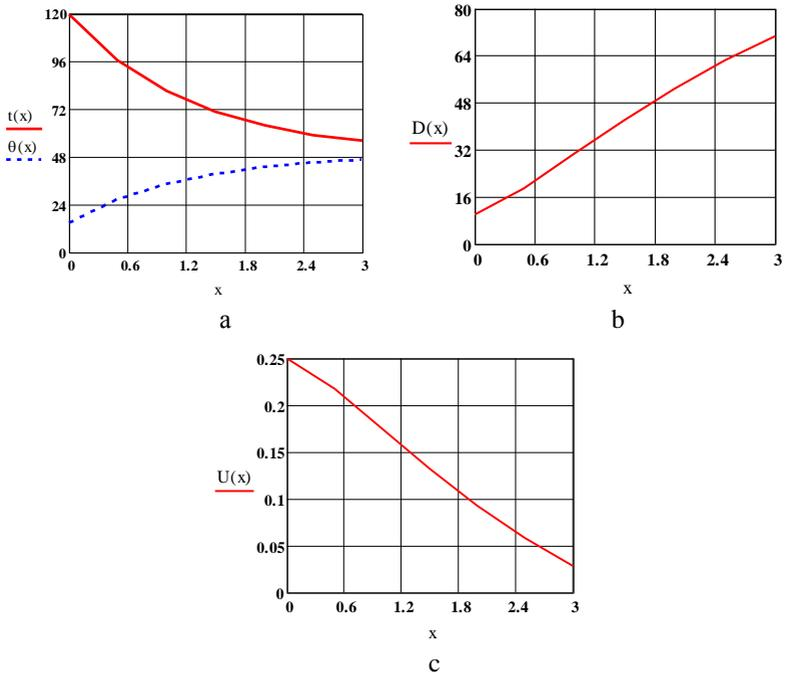
Fig. 2 — Changing grain parameters  $\theta$ ,  $U$  and drying agent  $t$ ,  $D$  the number of cycles (the length of the drying tract  $x = H_{\text{цикл}}$ )
