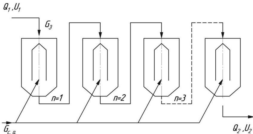
Fig. 1 — Diagram of the process of circulation dryers
